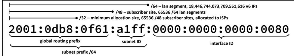
IPv6 addresses are written in hexadecimal and divided into eight pairs of two byte blocks, each containing four hex digits. Addresses can be shortened by skipping leading zeros in each block. This would shorten our example address to 2001:db8:f61:a1ff:0:0:0:80. Additionally, once per IPv6 IP, we can replace consecutive blocks of zeros with a double colon: 2001:db8:f61:a1ff::80.
